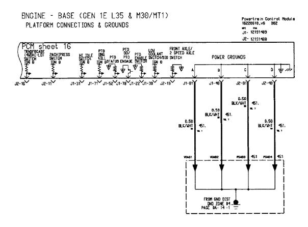
Figure 3.2.1a - XV - P/Truck - Mechanization Diagram - Power Distribution
